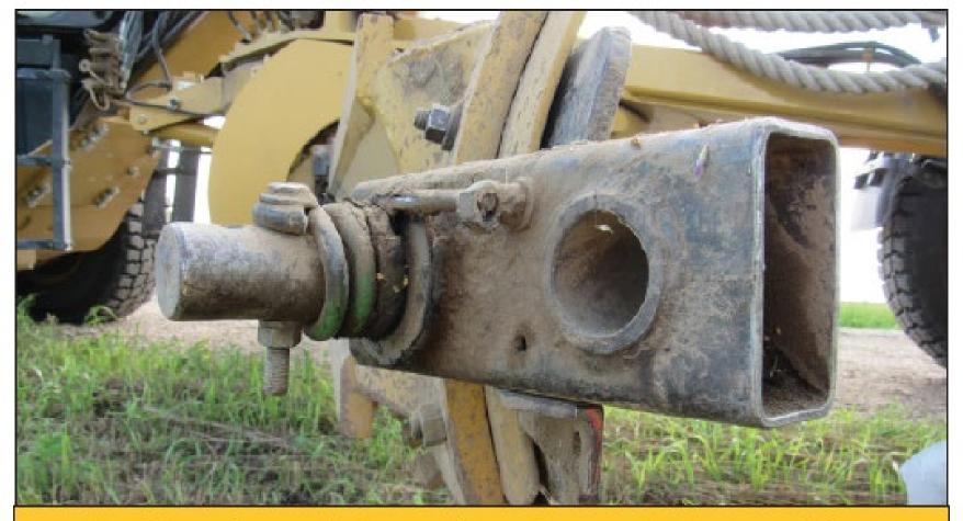
Spring Load Arm for Gravel Saver Disc
